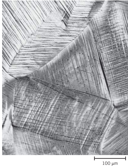
Figure 7.10 Slip lines on the surface of a polycrystalline specimen of copper that was polished and subsequently deformed. 173 \times .
