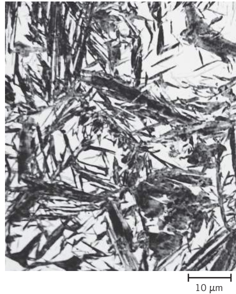
Figure 10.22 Photomicrograph showing the martensitic microstructure. The needle-shape grains are the martensite phase, and the white regions are austenite that failed to transform during the rapid quench. 1220 \times . (Photomicrograph courtesy of United States Steel Corporation.)
