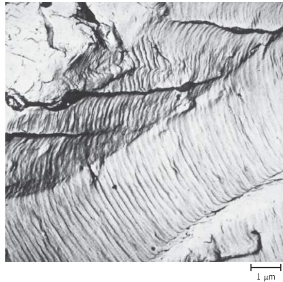
Figure 8.24 Transmission electron fractograph showing fatigue striations in aluminum. 9000 \times . (From V. J. Colangelo and F. A. Heiser, Analysis of Metallurgical Failures , 2nd edition. Copyright © 1987 by John Wiley & Sons, New York. Reprinted by permission of John Wiley & Sons, Inc.)
