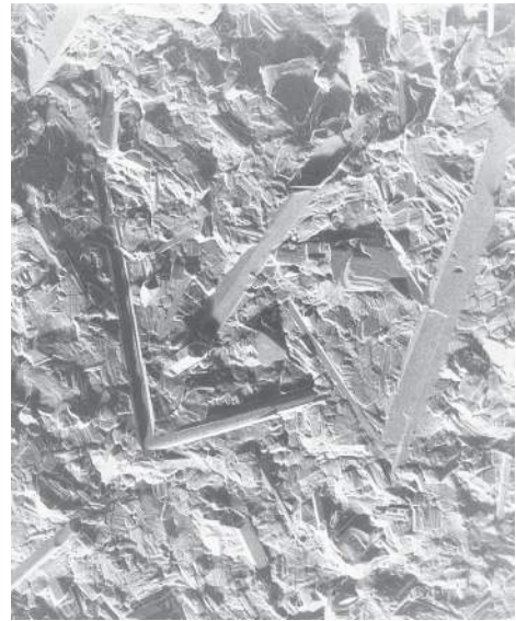
Figure 13.3 Scanning electron micrograph showing the microstructure of a glass-ceramic material. The long, acicular, blade-shape particles yield a material with unusual strength and toughness. 40,000 \times .
